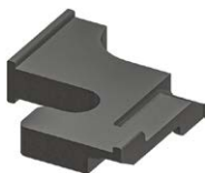
SK10-0030 Glass panel fixing/ stopping detail
